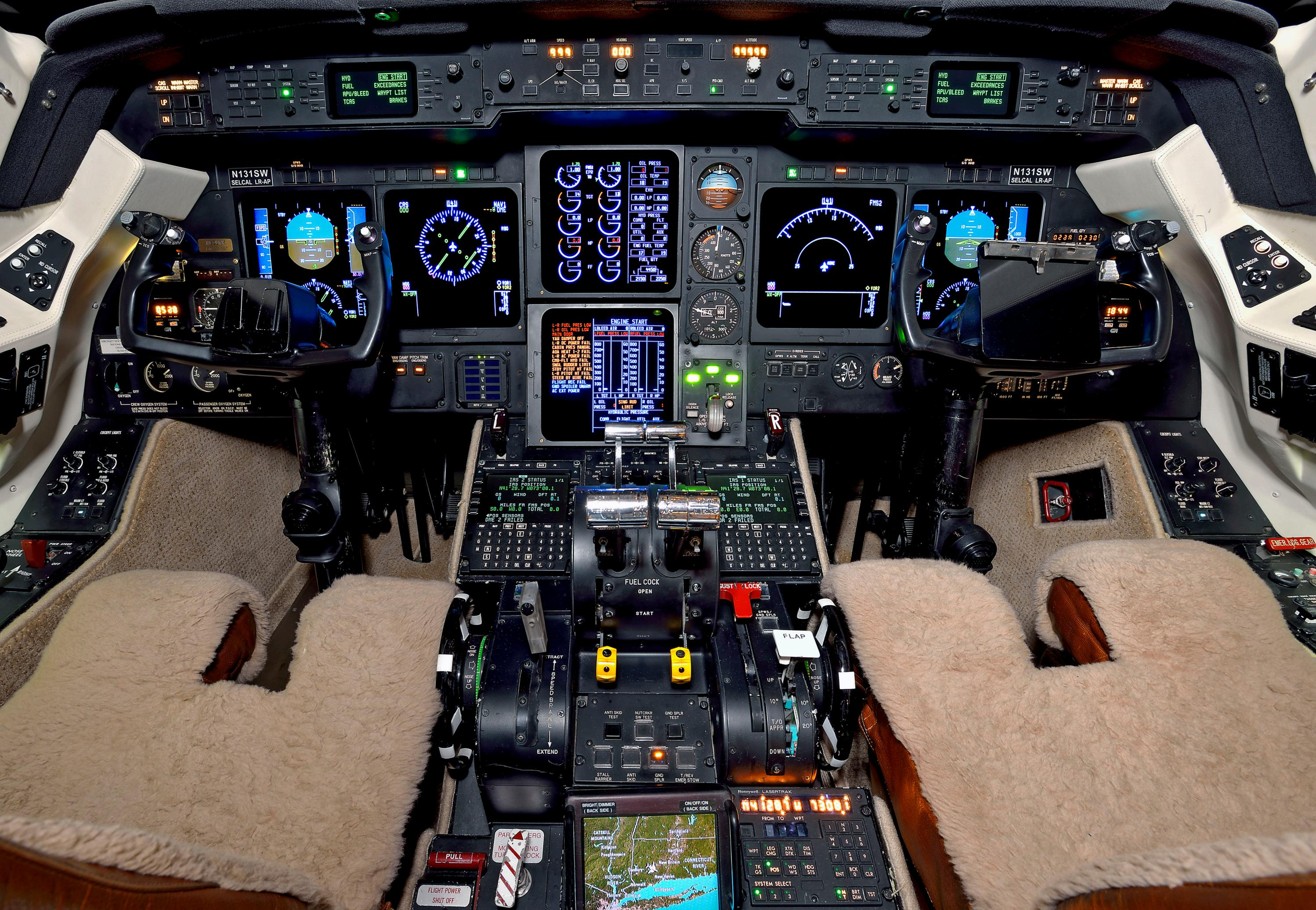
Top instrument panel with engine and system monitors. Left and right sides show 'HYD FUEL EXCEEDANCES' and 'APU/BLEED TCAS BRAKES' with 'ENG START' indicators. Central gauges include 'A/T MAN', 'SPEED', 'L NAV', 'HEADING', 'BANK', 'VERT SPEED', 'A/T', and 'ALTITUDE'. 'MASTER WARN CAS' and 'WIND SHIELD SCRLL' are also visible.
